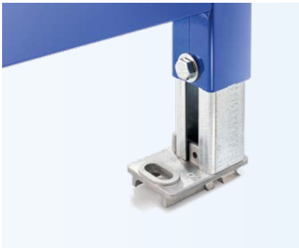
4 CLEVER FOOT PLATE DESIGN Thanks to a hollow space, the foot plate can also be mounted above the fastening screws on the floor profile without the screw head getting in the way.
