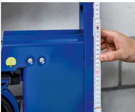
7 ADDITIONAL MARKINGS Markings on the blue frame make measuring easier for the centre of the threaded rod and middle of the connection bend.
