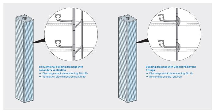
Performance comparison using the example of a residential building with 93 floors and 6.2 Discharge Units (DU) per floor.
